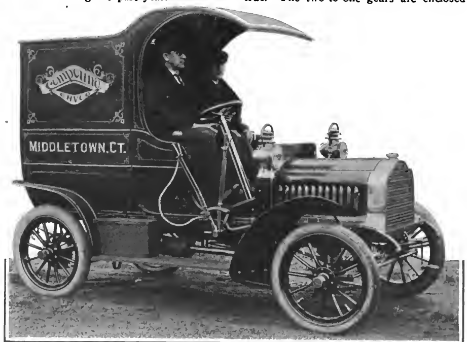
E. H. V. COMPOUND CAR FITTED WITH A LIGHT DELIVERY BODY.
